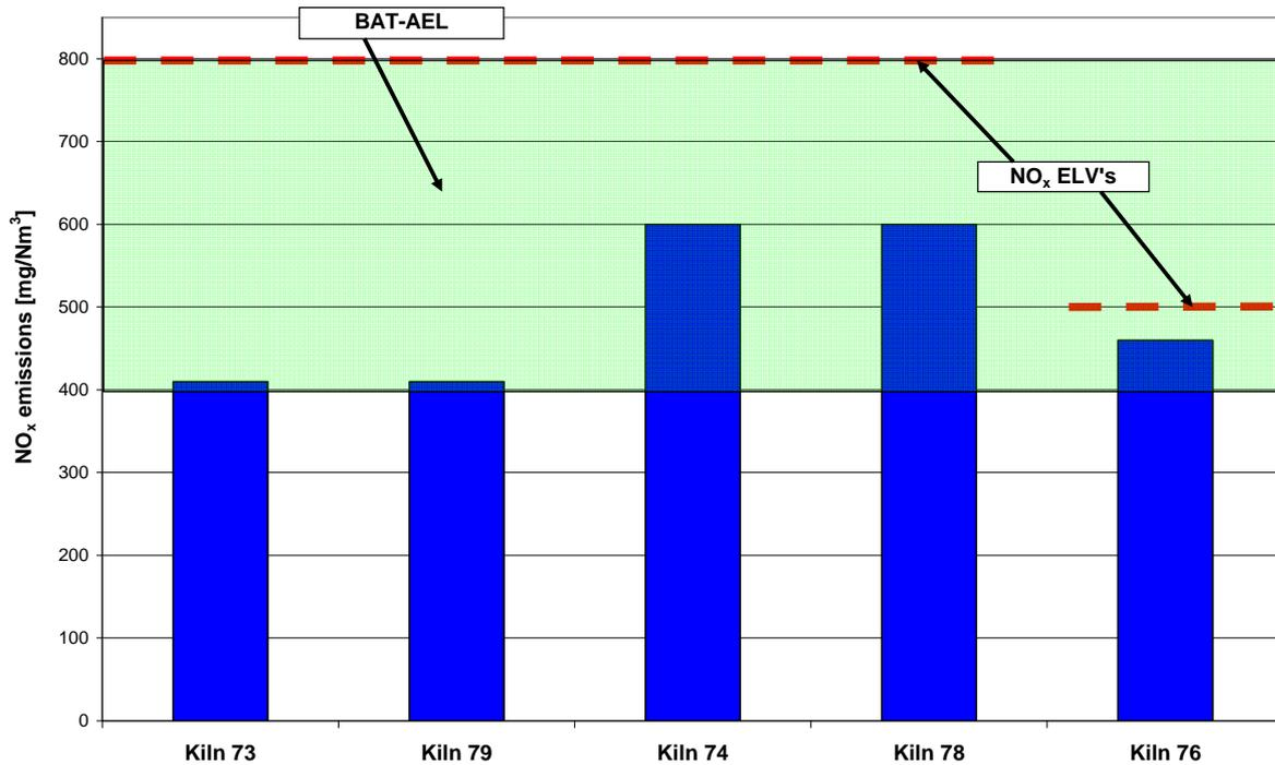
**Fig. 3:** Present NO<sub>x</sub> emissions of the white cement kilns (three stacks), BAT-AEL and NO<sub>x</sub> emission limit value
