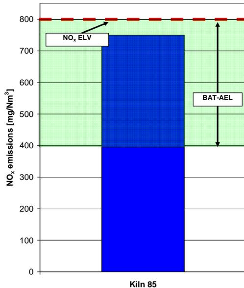
**Fig. 1:** NO<sub>x</sub> emissions from kiln 85
