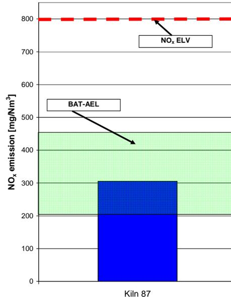
**Fig. 2:** NO<sub>x</sub> emissions from kiln 87
